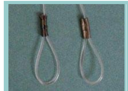
Left correct — note the uncompressed centre section and the flared ends of sleeve. Right incorrect — the sleeve has been compressed in the wrong direction damaging the monofilament
