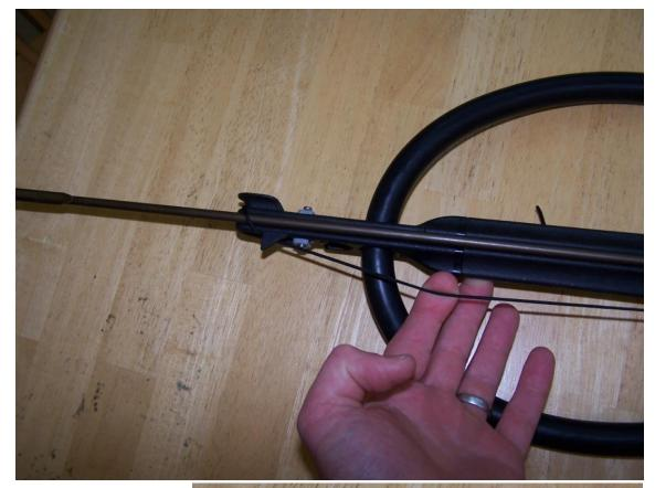
5. Line travels over shaft and down groove on other side. Holding shaft in place.
