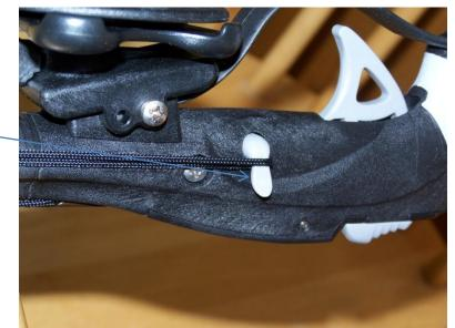
7. Line terminates at pin under the gun towards the barrel.
